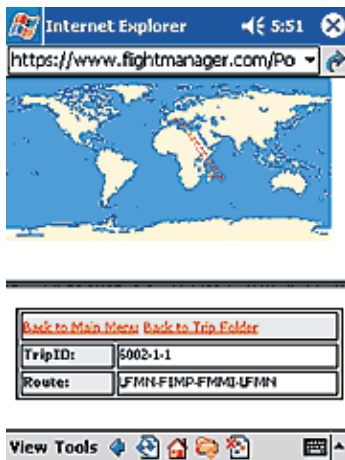
Fig. 4 (above). With ARI's Flight Manager and a Pocket PC, a pilot can view a specific flight route superimposed on an official aviation chart.
